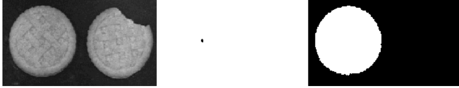
Figure 9: In respective order: the original, the marker (obtained by erosion), and the result (by reconstruction)
