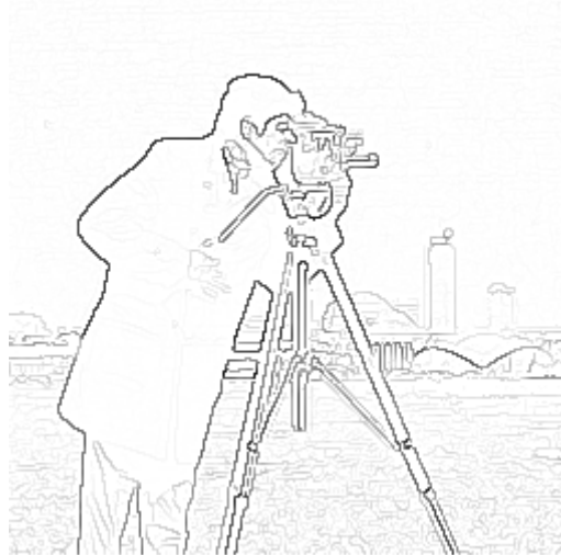
Figure 5: Canny edge detection with \sigma = 1 using thinning.
